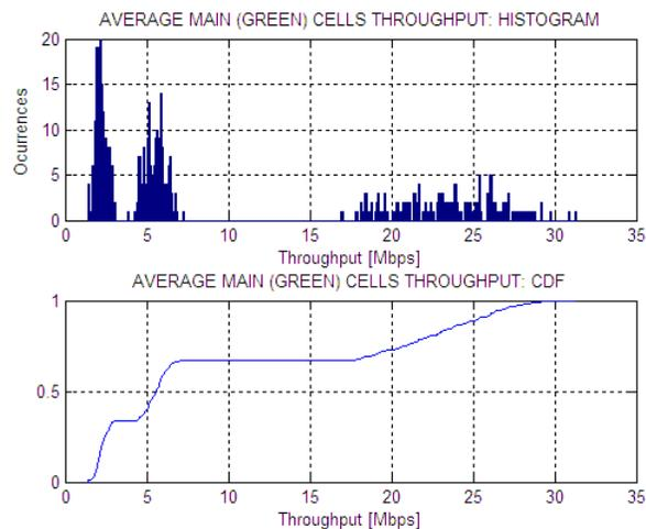
Fig. 5. Histogram and CDF of the DL average cell throughput (MIMO 2x2 with spatial multiplexing)
