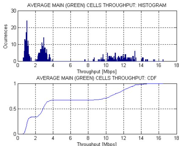
Fig. 4. Histogram and CDF of the DL average cell throughput (SISO)
