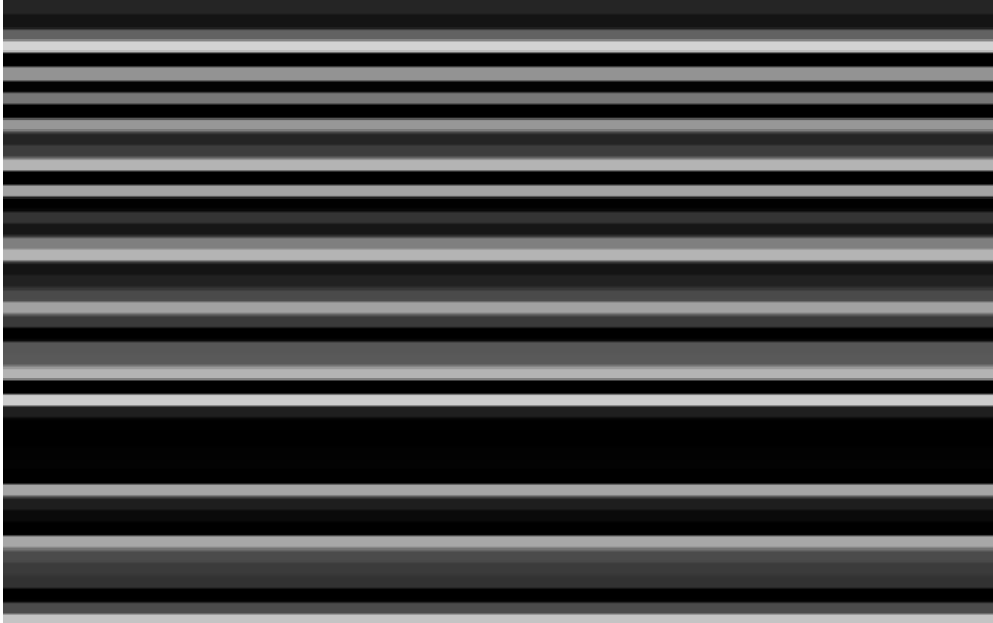
Figure 5.1: One realization of a confined stratified medium with 100 strata. Hydraulic conductivity is lognormally distributed; different greyscales denote different values of hydraulic conductivity.
