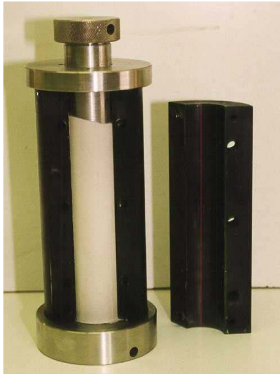
Figure 4.25 Silicone membrane inside the three-split fabrication mould.
