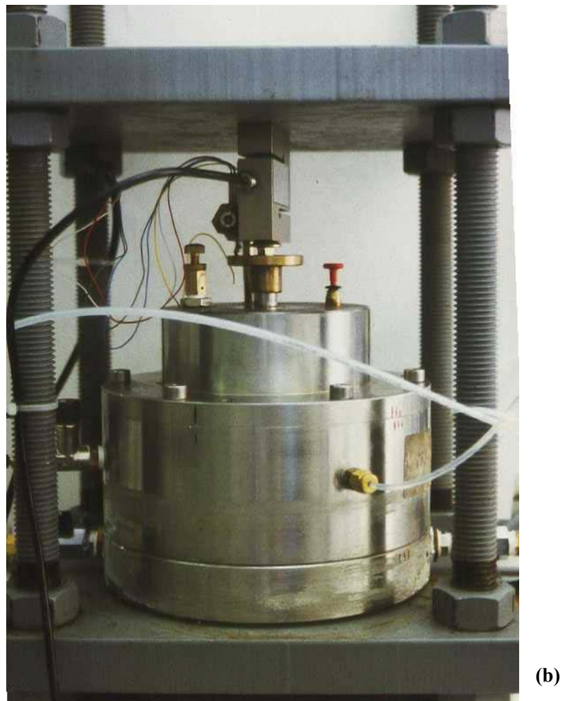
Figure 4.24 Layout of swelling pressure tests: a) thermal cell and b) lateral stress cell.
