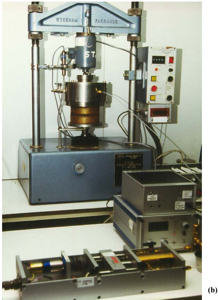
Figure 4.19 Experimental setup for static compaction tests: a) sample preparation in the hermetic mould inside the heating chamber, b) sample preparation in the lateral stress ring.
