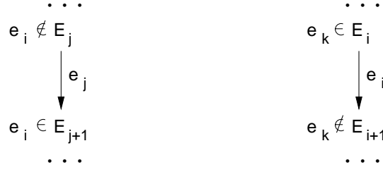
Figure 4.7 Enabling and disabling in a trace: (a) event e_j enables event e_i , and (b) event e_k is disabled by the firing of event e_i (the disabler).
