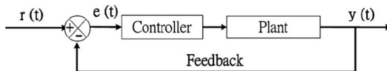
Fig. 1 Feedback Control system
