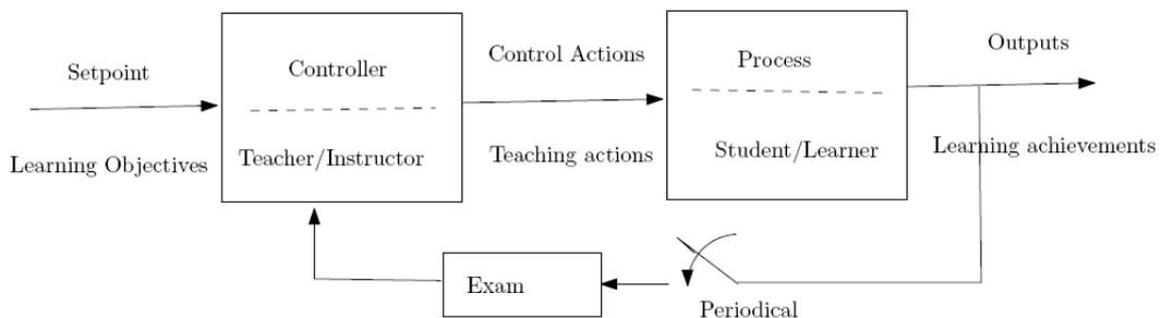
Fig. 3 Closed-loop instructional/control system
