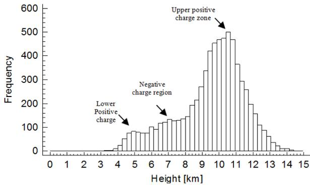
Figure 5- Median height distribution of the lightning sources (electrical charge distribution)
