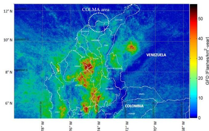
Figure 1 - Ground Flash Density at the north of Colombia derived from the Colombian LINET network. (Adapted from [14]).
