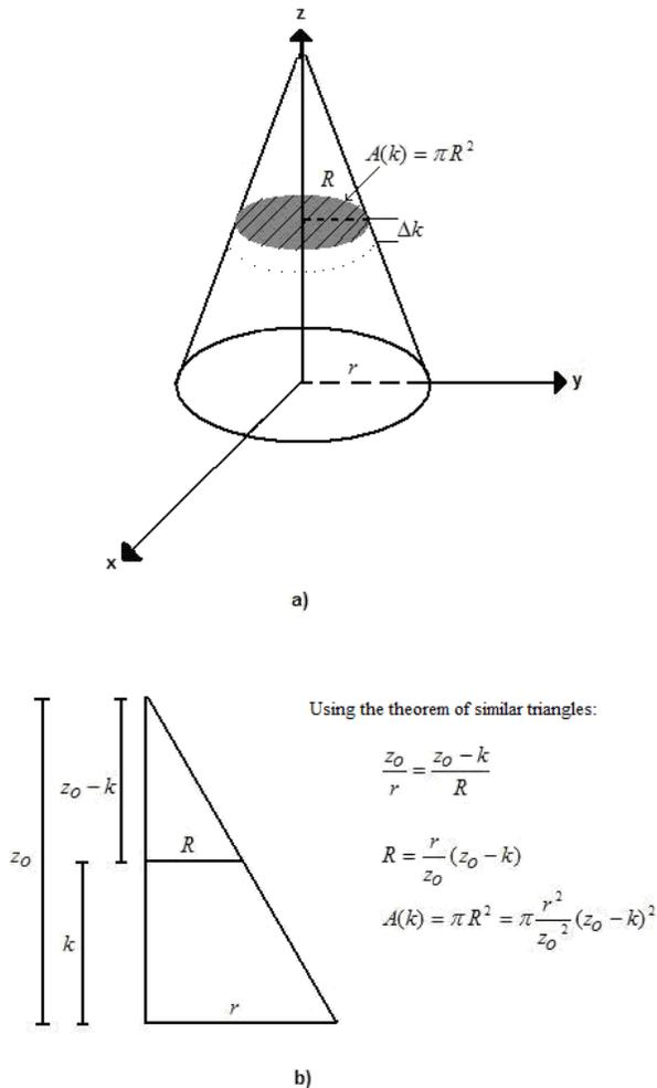
Figure 4. a) Area of the transversal section  $A(k)$  and the height differential  $\Delta k$ . b) Relationship between the radius  $R$  and the height  $k$  and system coverage area using the theorem of similar triangles.
