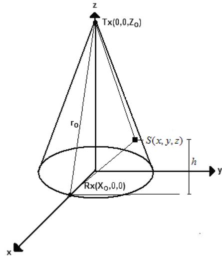
Figure 3. Spatial distribution of a fixed wireless communication system in presence of a scatter  $S$  delimited by a height  $h$ .
