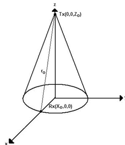
Figure 1. Spatial distribution of a fixed wireless communication system based on a HAP coverage area.
