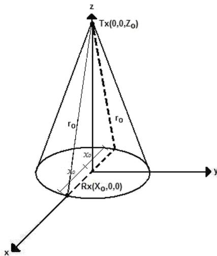
Figure 2. Maximum propagation path of a reflected wave  $K(\tau_m)$  (dotted line) depending on the geometry of the coverage area (cone) of the HAP system.
