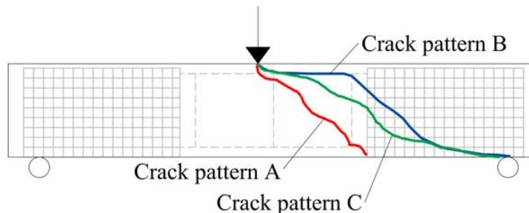
Figure 2. Crack patterns of tested beams.
