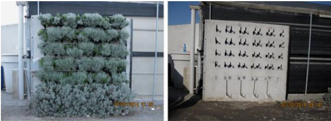
Figure 1. Experimental prototype with and without the modular greenery system
