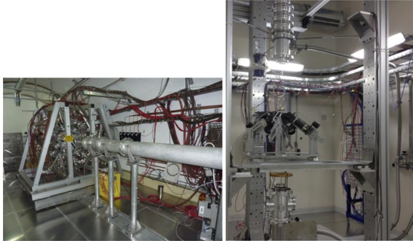
**Figure 3.** Total absorption calorimeter (TAC) in the n\_TOF-EAR1 (left panel) and C<sub>6</sub>D<sub>6</sub> scintillators set-up in n\_TOF-EAR2 (right panel). The horizontal and vertical beam lines are visible as well.
