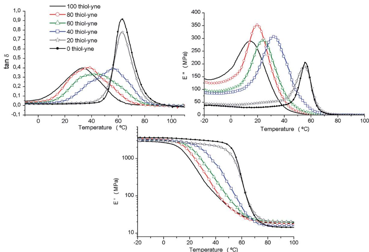
Fig. 4  $\tan \delta$  evolution, loss and storage moduli against the temperature for the materials obtained.
