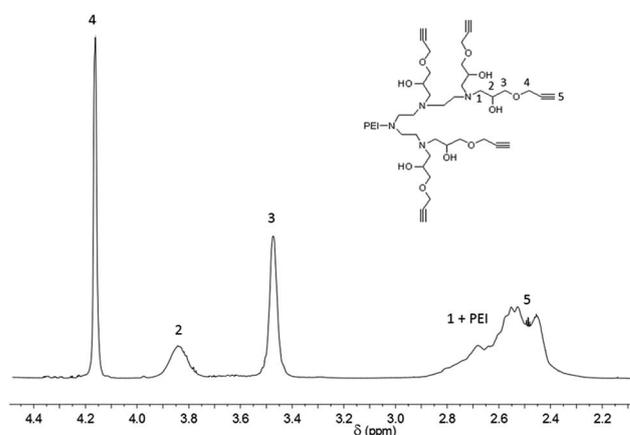
Fig. 1 <sup>1</sup>H NMR spectrum of propargyl-functionalized poly(ethyleneimine) PEIyne.
