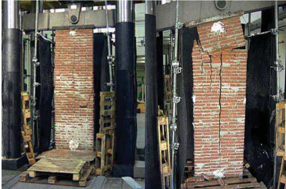
Figure 3. Break of the test number 7, with centred load (left), and 1, with eccentric load (right).
