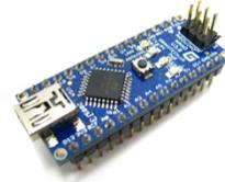
Figure 2: Arduino Nano microcontroller.
