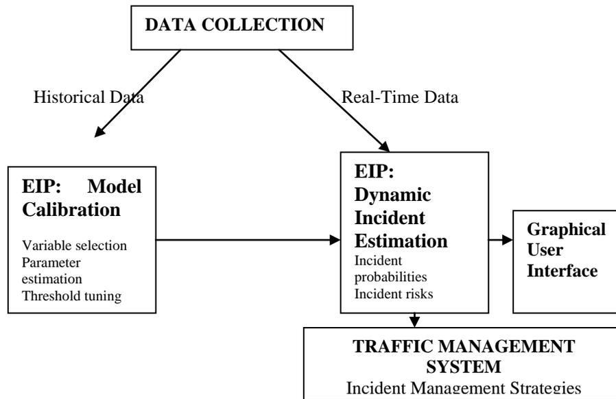
Figure 1. Estimation of Incident Probability Module in a Traffic Management System
