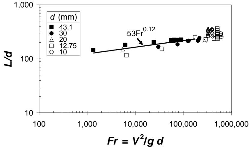
Fig. 1. Variation of normalized flame length as a function of Froude number: experimental results (subsonic and sonic velocity) and Eq. (2) (subsonic data).
