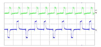
Fig. 5. Reception of PRK modulation: quench voltage (upper trace, 2 V/div) and differential voltage measured at the cross-coupled pair (lower trace, 500 mV/div). The time scale is 50 ns/div.
