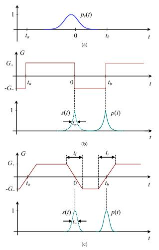
Fig. 2. (a) Input pulse. Conductance, sensitivity function and generated pulse: (b) in the step-controlled state; (c) in the slope-controlled state.
