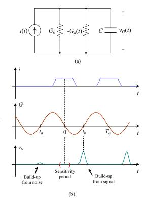
Fig. 1. (a) Basic RC circuit with variable conductance; (b) input signal, conductance and output voltage.
