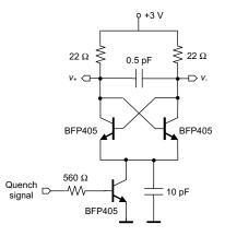
Fig. 3. Schematic of the implemented circuit.
