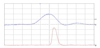
Fig. 4. Generation of a 0.5-ns pulse: quench voltage (upper trace, 0.5 V/div) and differential voltage measured at the cross-coupled pair (lower trace, 100 mV/div). The time scale is 1 ns/div.
