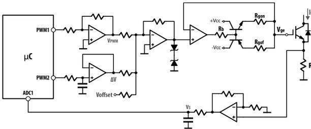
Fig. 12. Voltage adder circuit of the IGBT driver.
