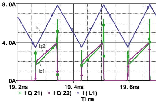
Fig. 10. Inductive current sharing in two parallel-connected IGBTs with balanced current sharing control based on the current average value control strategy.
