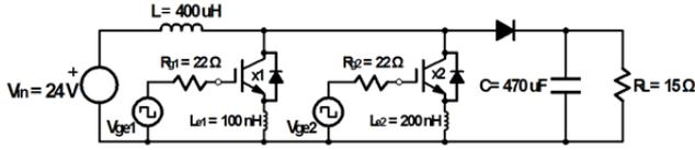
Fig. 2. Boost converter with a power switch based on two IGBT transistors connected in parallel.
