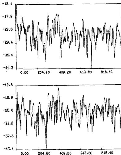
Fig. 7. Learning curves for neural filter (top) and linear Wiener filter (bottom).
