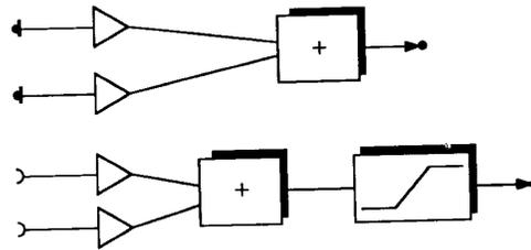
Fig. 1. Array beamformer (above) and neural model (below)
