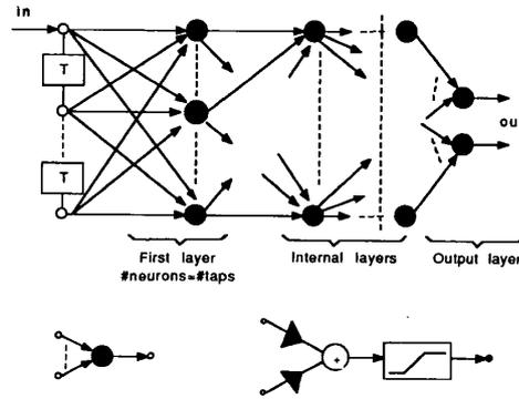
Fig. 5. Diagram of the generalized filter as a feed-forwards neural net.
