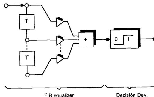
Fig. 3. FIR equalizer in a binary detection receiver and its similarity with a single neuron.
