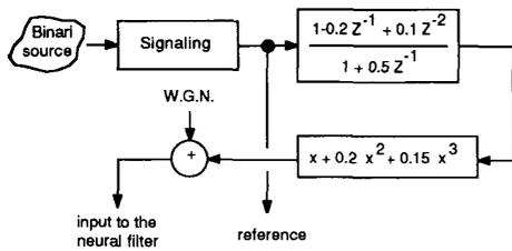
Fig. 6. Simulated communications environment to evaluate a neural filter with reference.
