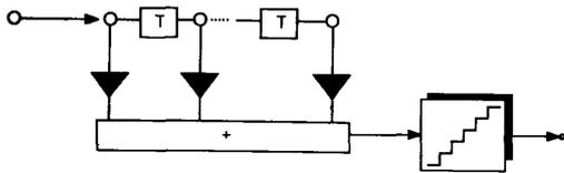
Fig. 4. A neuron as a FIR filter with A/D converter.
