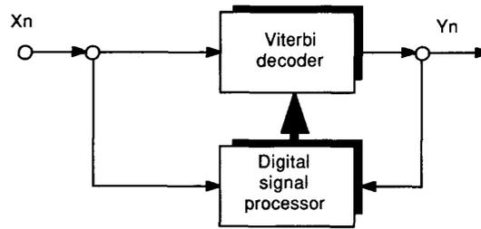
Fig. 2. Viterbi decoder with side information from a DSP.
