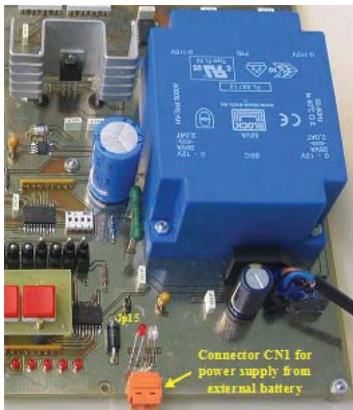
Fig. 2 Partial photograph that represents the power supply subsystem
