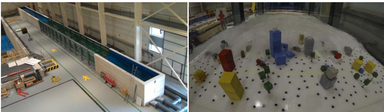
Figure 5. (a) Wave-Current Tsunami Flume (CoCoTsu) overview (b) Tsunami wave test
