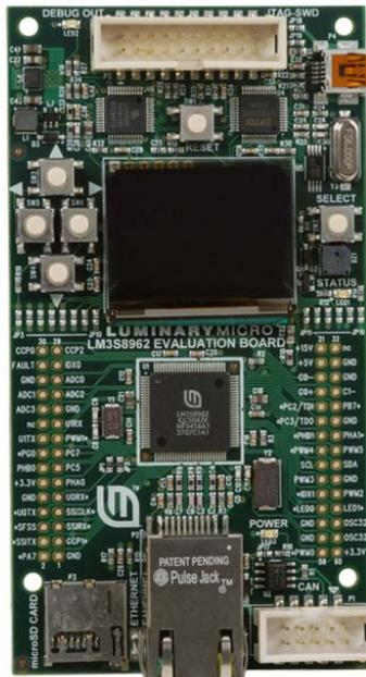
Figure 4: LM3S8962 Evaluation Board
