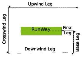
Figure 1. Aerodrome Landing Circuit
