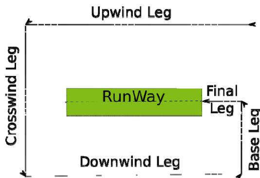
**Figure 1. Aerodrome Landing Circuit**
