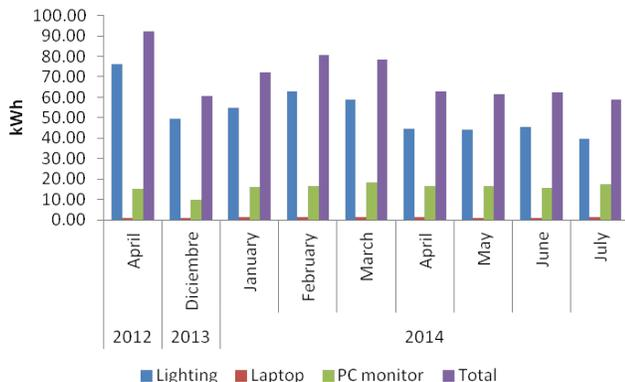
Fig 11. Power savings - smart lighting system
