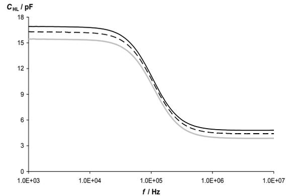
Fig. 7.  $C_{\text{HL}}$  measured for the cell with the first water sample (0,01 dS/m) at 52 mm (solid black line), 8 mm (dashed black line) and 1,7 mm (solid grey line) above the ground plane.
