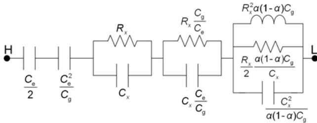
Fig. 2. Equivalent two-terminal impedance model for bipolar impedance measurements with capacitive electrodes.
