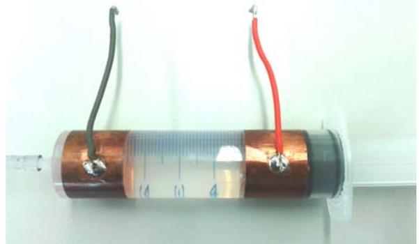
Fig. 3. Measurement cell with capacitive electrodes built from a polypropylene syringe and two copper rings.
