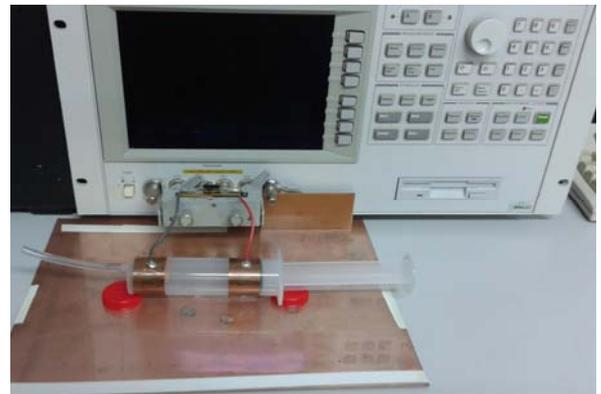
Fig. 4. Measurement setup with the cell placed over a ground plane and connected to the impedance analyser by single core cables.
