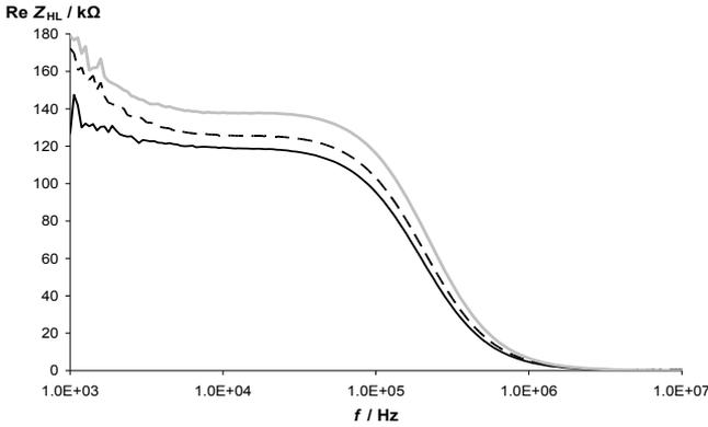
Fig. 5. Real part of  $Z_{\text{HL}}$  (0,01 dS/m) when the height of the cell above the ground plane was 52 mm (solid black line), 8 mm (dashed black line) and 1,7 mm (solid grey line).
