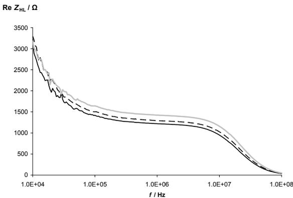
Fig. 6. Real part of  $Z_{\text{HL}}$  (1,0 dS/m) when the height of the cell above the ground plane was 52 mm (solid black line), 8 mm (dashed black line) and 1,7 mm (solid grey line).
