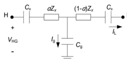
Fig. 1. Three-terminal lumped-parameter model for bipolar impedance measurements with capacitive electrodes.
