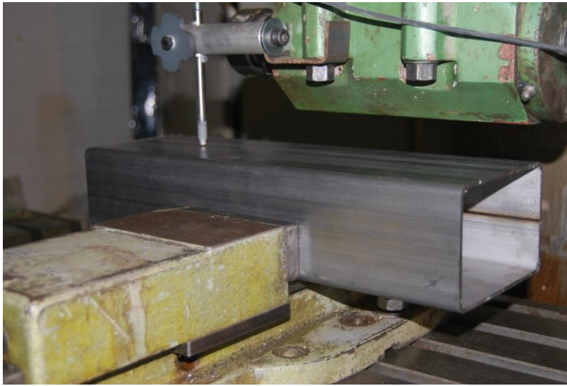
Figure 3. Setup for local geometric imperfection measurement.
