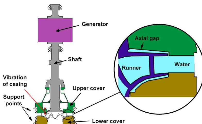
*Fig. 1. Runner nearby structures in a pump-turbine.*
