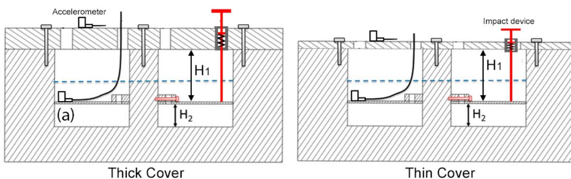
**Fig. 2.** Test rig cross section.
