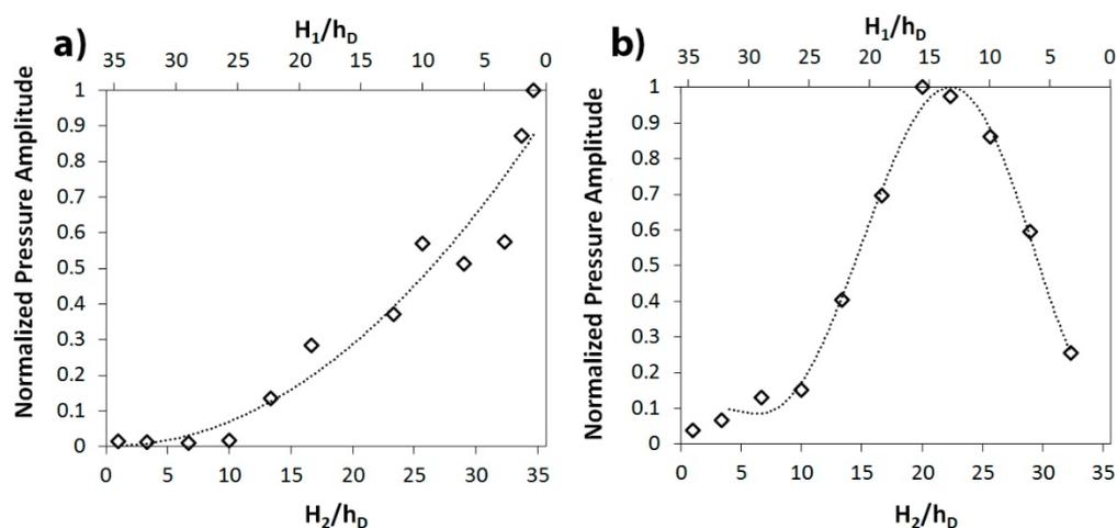
Fig. 6. Normalized pressure amplitude for a  $n=2$  and different distances to the covers. a) Thick cover. b) Thin cover.
