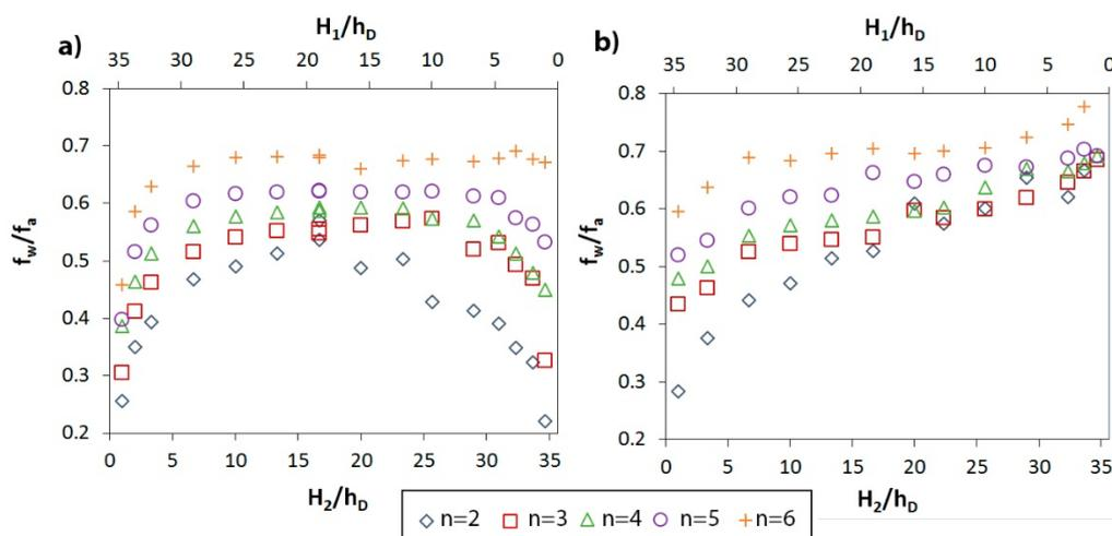
**Fig. 5.** Natural frequency in water ( $f_w$ ) over the natural frequency in air ( $f_a$ ) for different distances to the cover. a) Thick cover. b) Thin cover.
