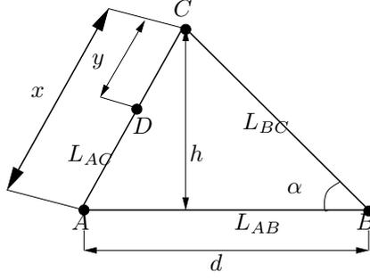
Figure 14: The general geometric constraint solving problem in 2D.
