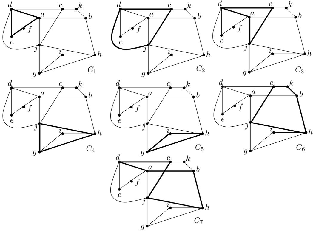
Figure 4: Fundamental circuits for the graph in Figure 3.
