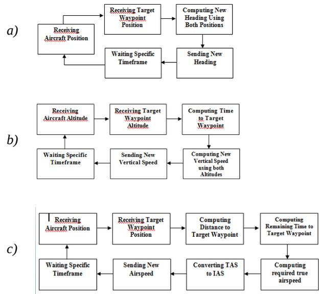
Figure 1 a) Heading Control, b) Altitude Control loops, c) Airspeed Control loops.
