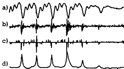
Fig. 2 Waveforms obtained in the proposed coder using a codebook of pulses. a) Synthesized signal. b) Original residual. c) Synthesized residual. d) Parametric envelope obtained with 10 parcors every 32 ms.
