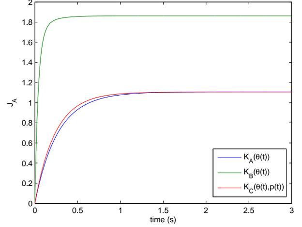
Fig. 1. Criterion  $J_A$  with the designed controllers.
