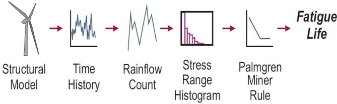
Fig. 1. Rainflow counting damage estimation procedure.
