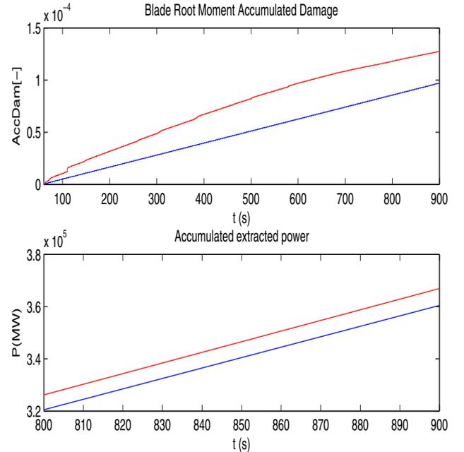
Fig. 6. Evolution of accumulated damages and accumulated extracted power with (blue) and without (red) health-aware objective in the MPC
