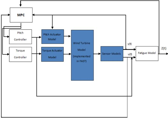
Fig. 5. Block diagram of wind turbine simulation and fatigue model
