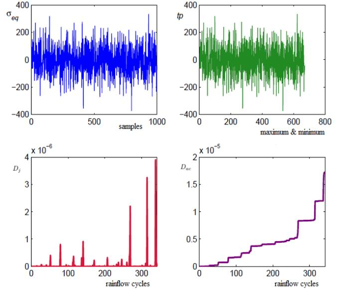
Fig. 2. Rainflow counting damage estimation procedure.
