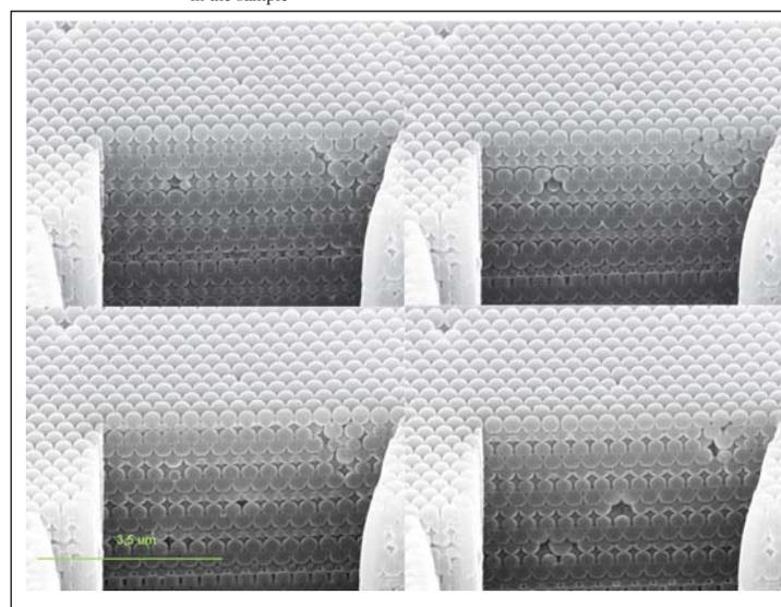
Fig.2. SEM images from the sample with 4 crosssections at 80nm distance
