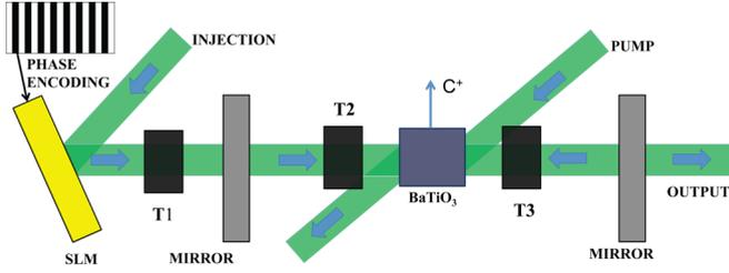
FIG. 1. (Color online) Sketch of the photorefractive oscillator with injected signal (rocking). Two mirrors form the resonator, which contains a BaTiO<sub>3</sub> crystal of  $4.5 \times 4.5 \times 8.0 \text{ mm}^3$ . SLM: spatial light modulator. T1, T2, T3: telescopic systems.
