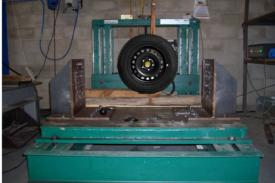
Apply the tyre a load not greater than 70% of the load index.
