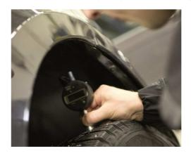
20 studs per tyre will be measured: 10 consecutive from both edges starting from a random point. More number of studs can be measured if there is a specific reason or is required by the applicant.
