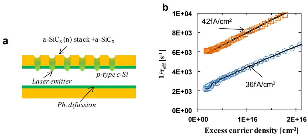
Fig 5. (a) Symmetrical test structure for measurements of minority carrier lifetime. (b) Determination of  $J_{oe}$  using the 'slope method' for a symmetrical sample before (blue round- shape) and after laser process (orange square-shaped) where a point-like selective emitter is created
