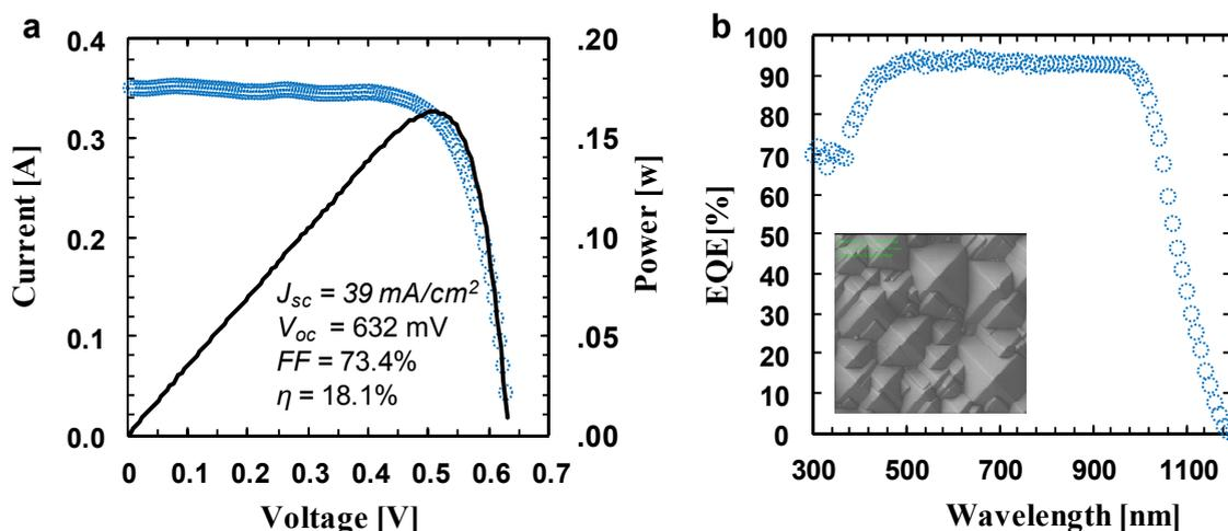
Fig 6.(a) I-V and P-V curves of the IBC cell with an area of 9 cm<sup>2</sup> and emitter coverage of 75%. Measurements under AM1.5G at 25 °C. Inset electrical parameters measured. (b) EQE vs. wavelength at 0.3 suns. A SEM image of random pyramids is shown in the inset.
