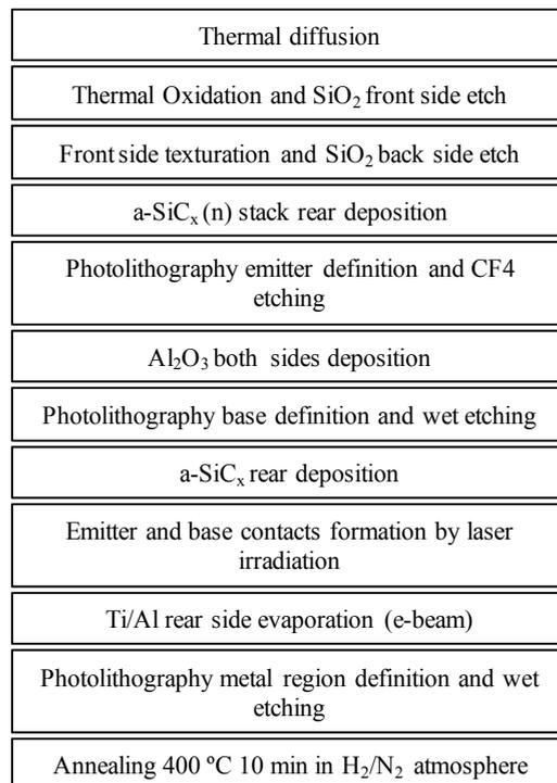
Fig 2. Fabrication process scheme IBC solar cell
