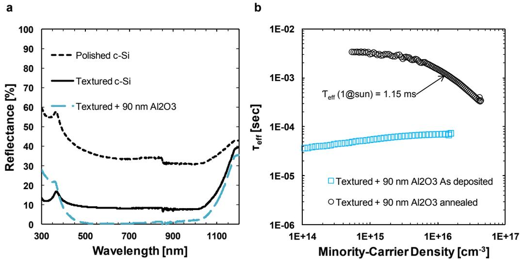
Fig 4.(a) Reflectance curves of 90 nm Al<sub>2</sub>O<sub>3</sub>-coated randomly textured c-Si (blue long dash), textured c-Si (black line) and bare polished c-Si as a reference (short dash); (b)  $\tau_{\text{eff}}$  vs. excess carrier density for symmetrical sample double-side textured and covered by 90 nm of Al<sub>2</sub>O<sub>3</sub> as-deposited and after annealing step.
