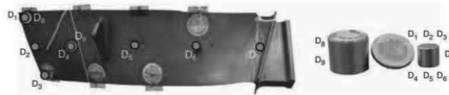
Figure 5. Locations of simulated damages
