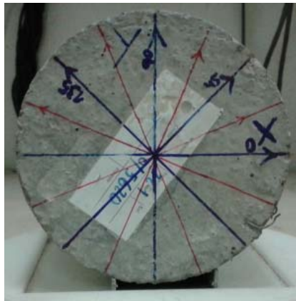
Figure 9. Axes of measurements in a cylindrical specimen
