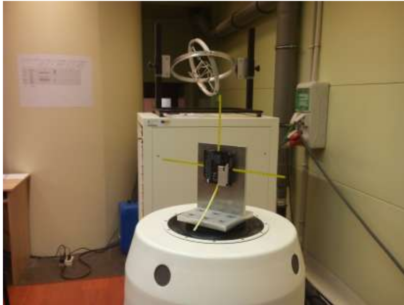
Fig. 11: Qualifying COMMS PCB on the NanoSat Lab shaker
