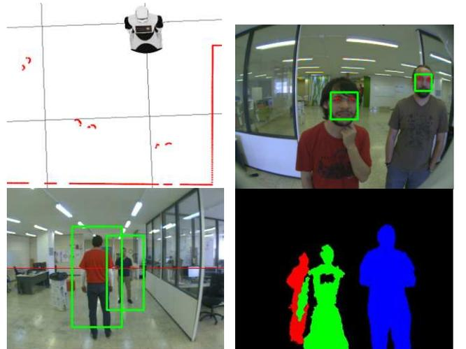
Fig. 5. Examples of detector outputs. Top-left: Clusters of points (in red) from a laser range scan showing typical human leg profiles. Top-right: Face detector. Bottom-left: Monocular body detector. Bottom-right: Skeleton detector.
