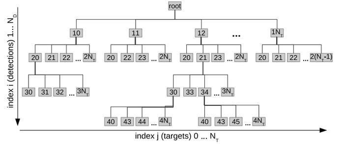
Fig. 3. Data association tree. The tree grows downwards driven by  $N_D$  detections, and sideways by  $N_T + 1$  targets. Target  $j = 0$  is the void target. In this figure, the tree is unfolded arbitrarily downwards due to space constraints of the paper, but horizontal unfolding shows how upper-level target indexes are skipped at each new down level, except for target  $j = 0$ .
