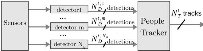
Fig. 2. Multi-target & multi-detector people tracking approach.
