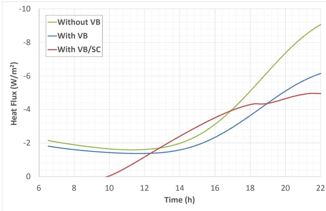
Figure 3: Heat flux through the inner wall for the studied DSF
