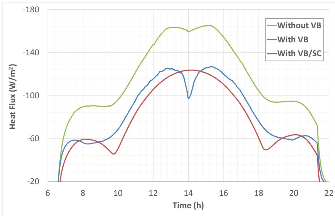
Figure 2: Heat flux through the inner glass for the studied DSF
