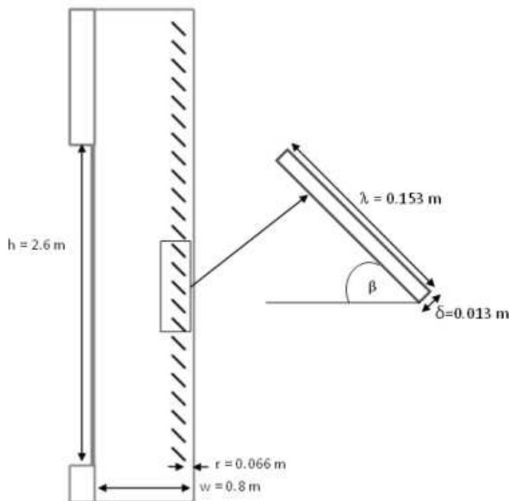
Figure 1. Geometric model used
