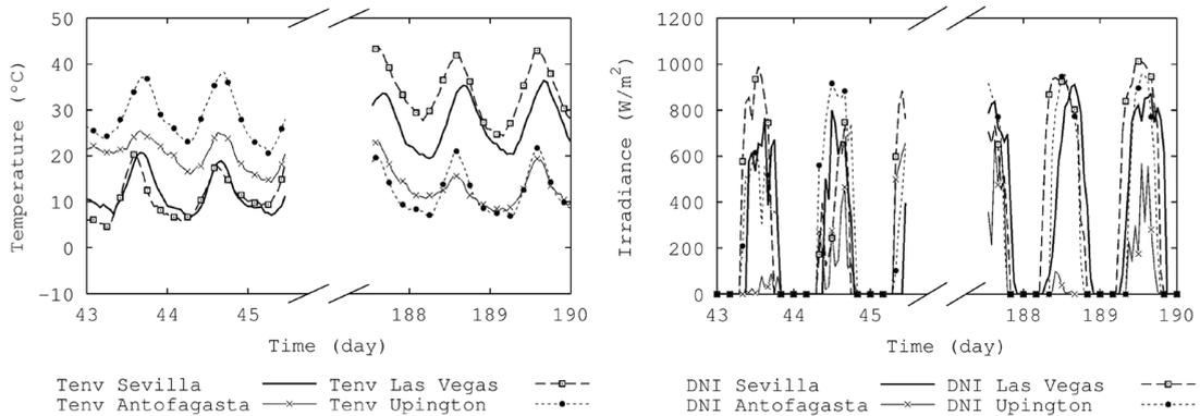
Fig. 4. Boundary conditions of the storage tank system (for different locations). Input data: (left) Ambient temperatures; (right) Direct normal irradiation.
