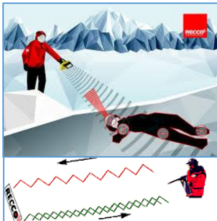
Figure 41: signal diagram RECCO system
