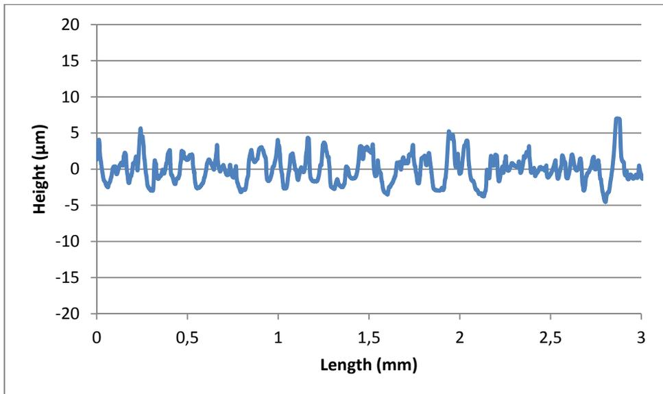
**Figure 6** Roughness profile for an experiment with  $GS=91$ ,  $DE=30$ ,  $PR=400 \text{ N/cm}^2$ ,  $VL=$  and  $VT=...$
