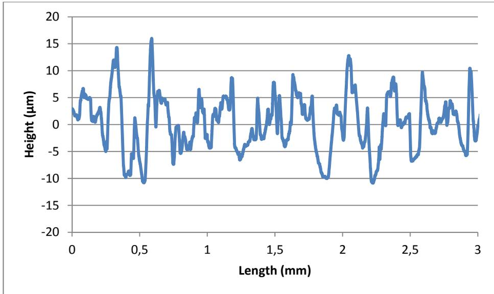
**Figure 5** Roguhness profile for an experiment with  $GS=181$ ,  $DE=60$ ,  $PR=700 \text{ N/cm}^2$ ,  $VL=$  and  $VT=...$
