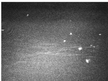
Fig. S3. BAM image (3.6 mm x 4.1 mm) for a lipid-containing artificial tear extended on water.
