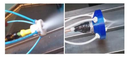
Fig. 2. Proposed nozzle adapter.
