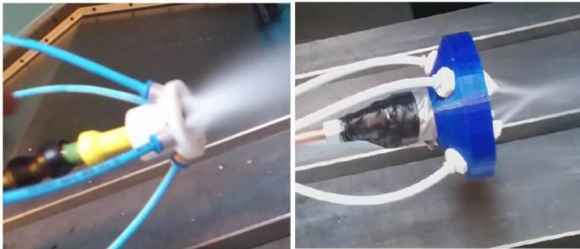
Fig. 2. Proposed nozzle adapter.
