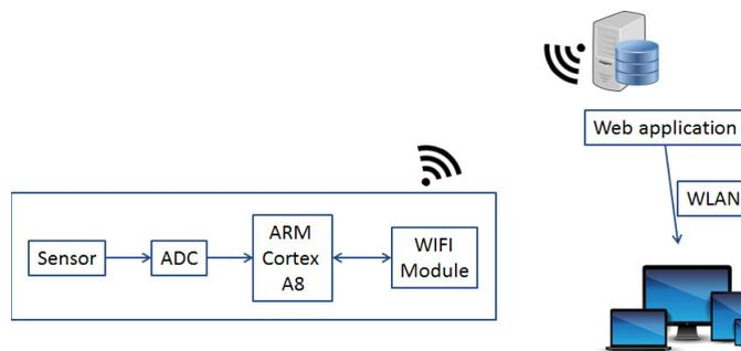
Fig 1. Conceptual architecture of the data acquisition system
