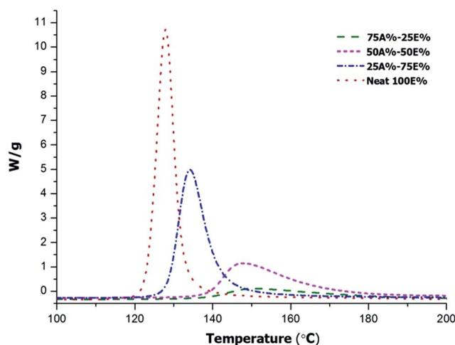
Fig. 2 Dynamic DSC thermograms at 10 °C min<sup>-1</sup> of non-irradiated thiol-ene/thiol-epoxy mixtures with different proportions of epoxy and allyl compounds.
