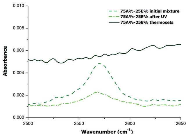
Fig. 4 FTIR region corresponding to S–H stretching absorption band for the formulation with 75% of thiol-ene of the initial mixture, after irradiation and after complete curing.
