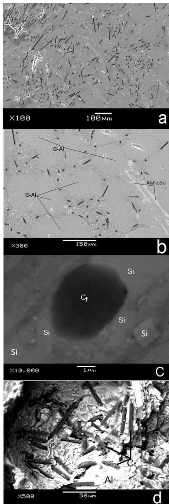
Fig. 2 Microstructure of successful A356/ $C_{sf}$  composite showing random orientation of fibers in the aluminum matrix (a)  $\times 100$ , (b)  $\times 300$ , microstructure of interface of  $C_{sf}$  and aluminum matrix (c), Fractured surface of composite which shown fibers in matrix (d)
